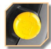
Lumbar adjuster control (continuous mechanical adjustment)
